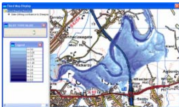
Example of the flood map display in Delft -FEWS, showing floodplain flooding in a 14km reach of the Eden River, Northwest Region, UK (reproduced by kind courtesy of the Environment Agency, UK)
