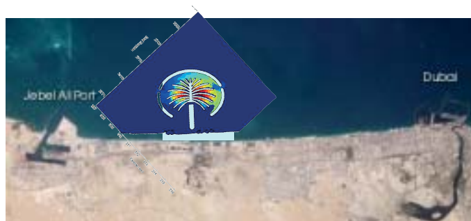
Figure 6: Numerical modelling was undertaken to investigate the flushing of the Palm Island scheme and to assess the impact of the land reclamation on the seabed and coastline.
