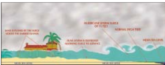
Effect of a storm surge along the coast (courtesy NCstormsurge.com)
